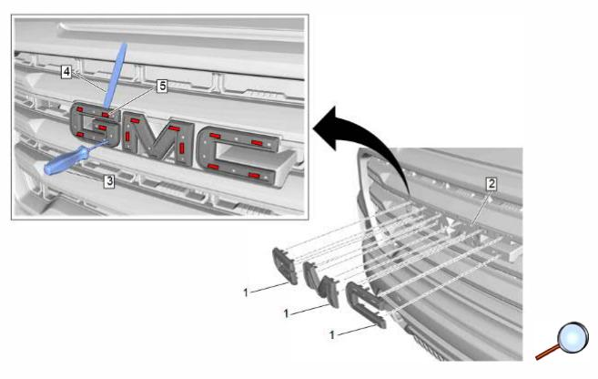
5. Using a suitable small flat bladed tool (3), carefully disengage the retention tabs (5) while using a suitable plastic flat-bladed tool (4) behind the each letter bezel while pushing forward and remove each letter (1) from grille (2). Be careful to avoid damage to the retaining tabs in the grille (2), as this may result in loose fit of the new emblems.
