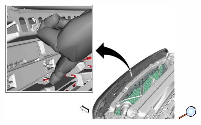
9.8. Make a gap between the front grille and aero shutters by slowly pulling front grille forward and reaching down with hand to the emblem tabs (1) one by one and gently move any non-engaged tab up/down or left/right, depending on tab orientation, until the tab is fully seated or unless you hear an audible click sound of tab being engaged.
