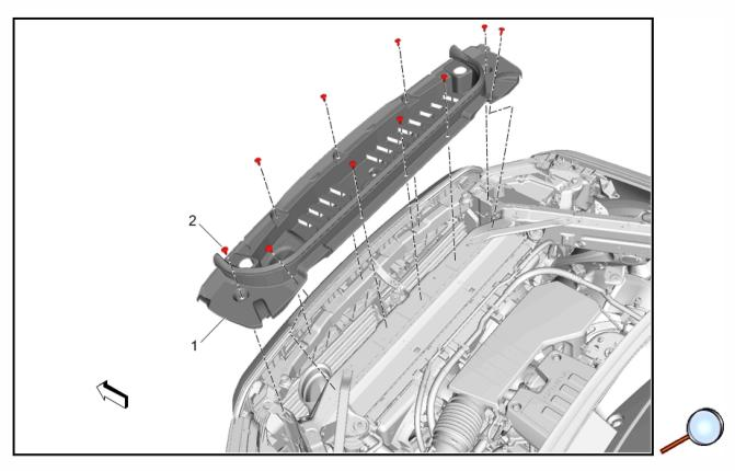
9.12. Re-install the front compartment front sight shield (1) and the previously retained front compartment front sight shield push-in retainers (2).
