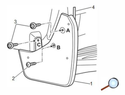
5. Making sure that the tape pull tab (4) is visible, place splash guard (1) to the vehicle taking care to remove any gaps to the vehicle.
