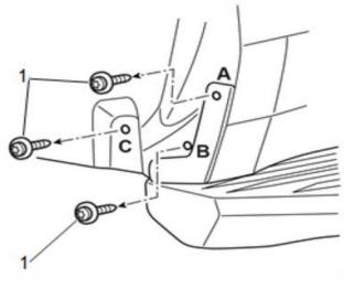
4. Remove existing screws (1) at locations (A), (B) and (C). Retain screws at (A) and (C) and discard (B).
